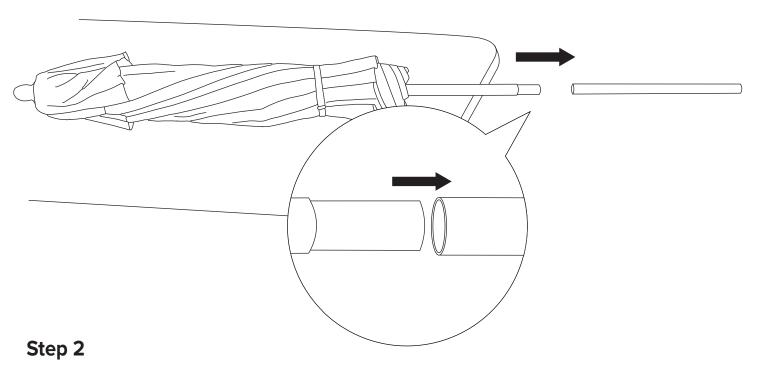
Twist the bottom pole clockwise to thread the screw into the hole of the frame.
