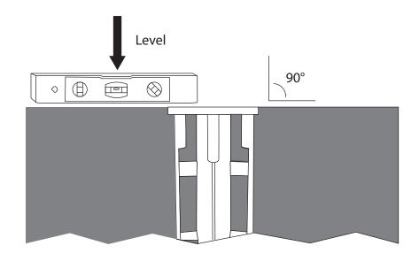
**Step 6**After the concrete has cured, remove our bolts from the threaded holes of the Ground Anchor.
